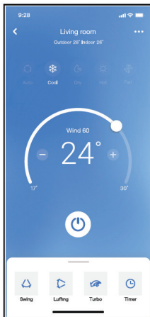
fig. 25 - Thus, user can control air conditioners on/off status, operation mode, temperature, fan speed and so on.
